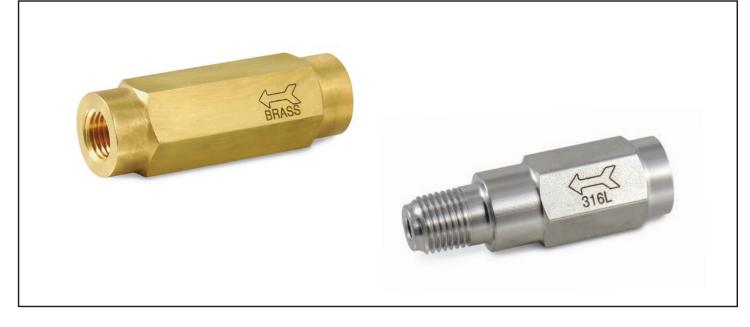
GasFlo Products CV-BS Series Check Valves prevent the reverse flow of gas/fluids and protects regulators, cylinder valves, purge assemblies and manifold systems. Manufactured from bar stock this poppet and spring design with an 0-ring at the valve seat ensures positive shut off and quick acting response.
