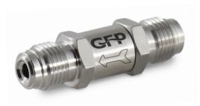
GasFlo Products CV-SB Series Check Valves provide easy in-line installation to prevent the reverse flow of gas/fluids in analytical and high-purity assemblies. A two-piece split body poppet and spring design with an 0-ring at the valve seat ensures positive shut off and quick acting response.
