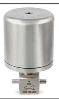
GasFlo Products HPSL Series Valves are air operated to allow for remote automated cycling. This high pressure springless diaphragm design is available in normally closed or normally open configurations. Valve remains in a static state unless proper actuation pressure is continuously applied. HPSL Series Valves provide superior leak integrity for critical gas/fluid systems with pressure ranges from vacuum to 3500 psig.
