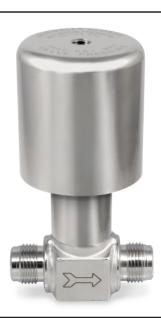
GasFlo Products HPST-8 Series Valves are air operated to allow for remote automated cycling. This high pressure, forged body, spring type diaphragm design is available in normally closed or normally open configurations. Valve remains in a static state unless proper actuation pressure is continuously applied. HPST-8 Series Valves provide superior leak integrity in 3/8" and 1/2" applications with pressure ranges from vacuum to 3500 psig.
