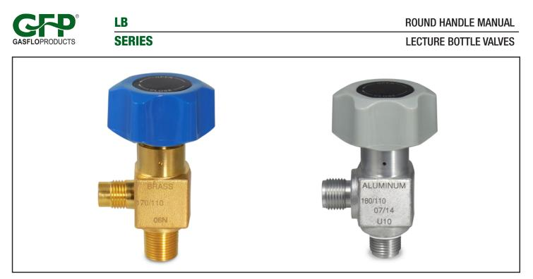
GasFlo Products LB Series Lecture Bottle Valves provide a positive shut off for Lecture Bottle Cylinders and other small gas cylinder applications. This economical spring type, diaphragm, forged body valve offers superior leak integrity and precision machined NGT and UNF inlet threads. Cleaned for O<sub>2</sub> service, GFP LB Series Valves are the perfect choice for all specialty and medical gas packages.
