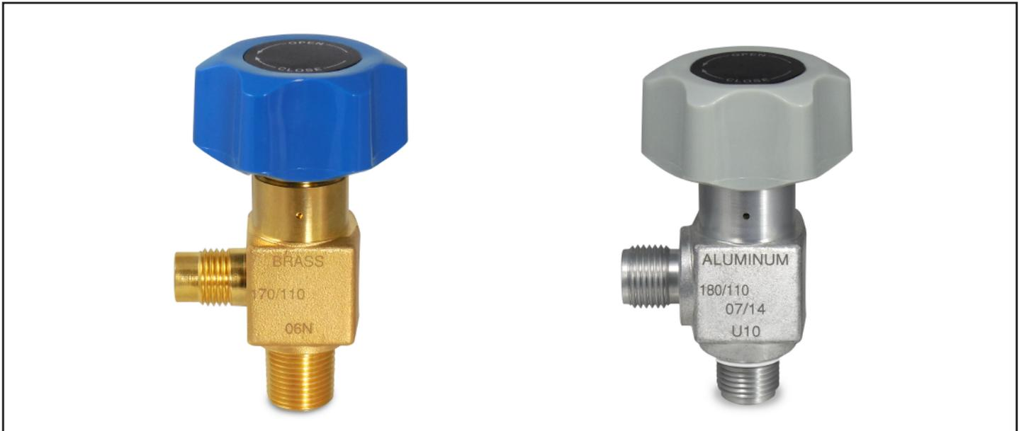
GasFlo Products LB Series Lecture Bottle Valves provide a positive shut off for Lecture Bottle Cylinders and other small gas cylinder applications. This economical spring type, diaphragm, forged body valve offers superior leak integrity and precision machined NGT and UNF inlet threads. Cleaned for O<sub>2</sub> service, GFP LB Series Valves are the perfect choice for all specialty and medical gas packages.
