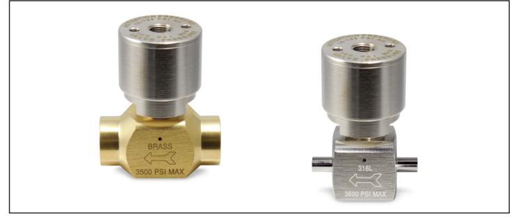
GasFlo Products LPSL Series Valves are air operated to allow for remote automated cycling. This low pressure springless diaphragm design remains closed unless proper actuation pressure is continuously applied. LPSL Series Valves provide superior leak integrity for critical gas/fluid systems with pressure ranges from vacuum to 150 psig.
