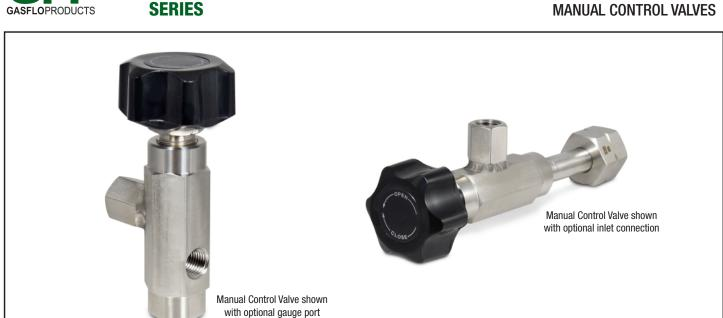
GasFlo Products MC Series Manual Control Valves provide a positive shut off direct from a cylinder valve outlet when a regulator is not required. This packed type design is suitable for high pressure applications (3000 psig max) and offers basic flow metering capability. Available with a specified cylinder connection inlet and gauge port on request.
