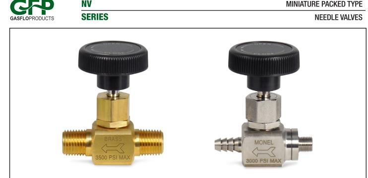
GasFlo Products NV Series Packed Type Needle Valves provide a positive shut off and basic flow metering capability. Available in lecture bottle control, angle, and in-line control configurations, these miniature valves are machined from bar stock and are suitable for high pressure applications.
