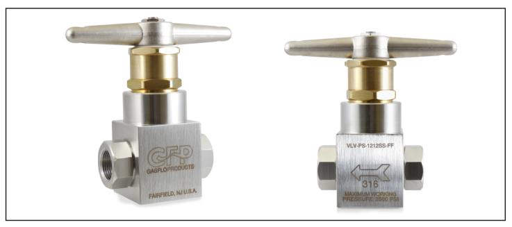
Originally designed for BF3 service, this GasFlo Products Pressure Seal Valve has proven to be a valuable addition for all high pressure compressed gas manifolds. Used as a master shut-off valve, the pressure seal design assures a positive seal: the higher the service pressure, the better the seal. The large tee bar handle allows for easy operation under heavy back-pressure conditions. With a high flow coefficient (Cv = 3.5) this valve is ideal when large volumes of product are required.
