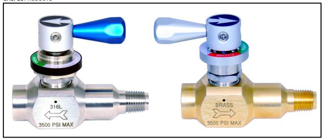
GasFlo Products QLL Series Valves are manufactured with an extended inlet leg and provide quarter turn, positive shut off for critical gas/fluid systems. The Lever handle and multi port collar design allows for visual open/closed indication and simple lever reorientation when required. This springless diaphragm valve offers superior leak integrity for Specialty Gas, Chemical, Instrumentation, Semiconductor, Medical and general purpose applications with pressure ranges from vacuum to 3500 psig.
