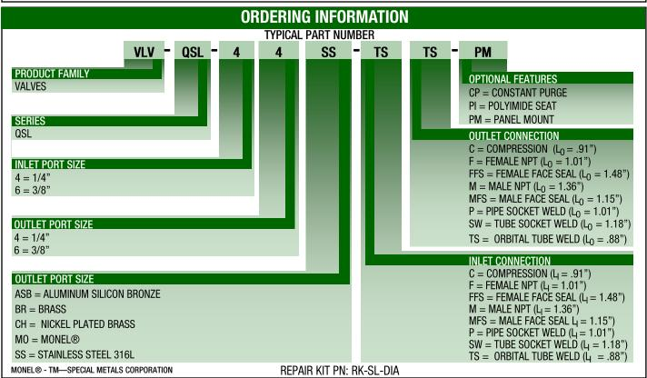
3 PORT, 4 PORT AND CUSTOM CONFIGURATIONS ARE AVAILABLE ON REQUEST. ALSO AVAILABLE WITH PNUEMATIC OPERATOR, SEE LPSL AND HPSL SERIES. Minimum order quantities may be required. Some inlet/outlet combinations may not be available.
