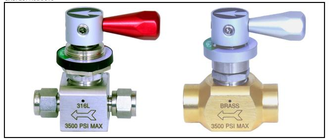
GasFlo Products QSL Series Valves provide quarter turn, positive shut off for critical gas/fluid systems. The Lever handle and multi port collar design allows for visual open/closed indication and simple lever reorientation when required. This springless diaphragm valve offers superior leak integrity for Specialty Gas, Chemical, Instrumentation, Semiconductor, Medical and general purpose applications with pressure ranges from vacuum to 3500 psig.
