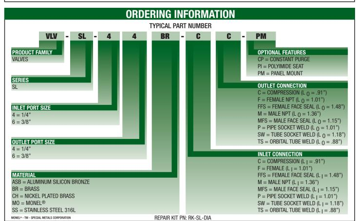
3 PORT, 4 PORT AND CUSTOM CONFIGURATIONS ARE AVAILABLE ON REQUEST. ALSO AVAILABLE WITH PNUEMATIC OPERATOR, SEE LPSL AND HPSL SERIES.
