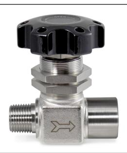
GasFlo Products ST-8 Series Valves are a high pressure, medium flow design. This spring type, diaphragm, forged body valve can be easily field maintained with an economical re-build kit. The ST-8 Series provides an extended service life, positive shut off and smooth operation in 3/8" and 1/2" applications with pressure ranges from vacuum to 3500 psig.
