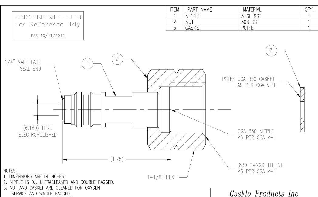
4. ASSEMBLY IS BULK BAGGED AND LABELED WITH GFP LOGO AND GFP PART NUMBER.
